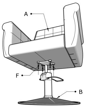
Then attach seat to the assembled bracket and hydraulic.
